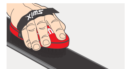
5: Brush firmly with the Steel Brush (T0179 or T0162). The ski is now ready for application of new glide wax.
