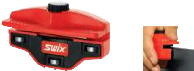
TA3008 SWIX PHANTOM R EDGE FILE HOLDER Economy edge sharpener with ball bearings and 80 mm file. Easy adjustment from 85 to 90 degrees. Ergonomic, longer holder for stability and good grip. Protects the hand. Takes files and stones up to 6 mm thickness. Easy tightening of files.
